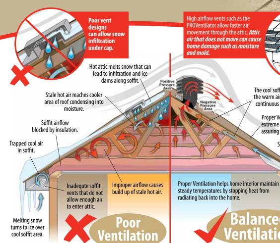
High airflow vents such as the PROVentilator allow faster air movement through the attic. Attic air that does not move can cause home damage such as moisture and mold.
