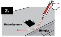
2. Using a 1/2 inch bead, apply a generous amount of construction sealant to the underlayment infront of hole before applying next shingle course.
