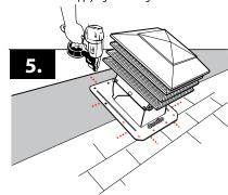
5. Position the roof vent over the cut opening in the roof. Center the vent by aligning edges of the vent throat with the chalk lines previously marked. Using the molded nail indicators, nail the top half of the vent securely into place.
