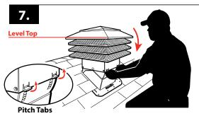
7. Using the pitch tabs lower the top of the unit back to desired pitch. Ensure the top of the unit is level.
