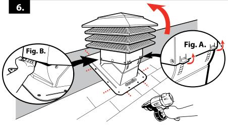
6. Gently lift the pitch calculating tabs (Fig A.), rotating the top of the unit up to make room for nailing the bottom half of the flange (Note: Ensure the vent throat overlaps (Fig B.). Using the molded nail indicators, nail the remainder of the vent securely into place.
