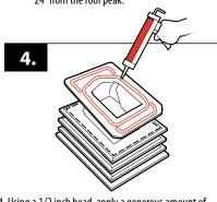
4. Using a 1/2 inch bead, apply a generous amount of construction sealant to the base of the vent.
