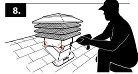
8. Using the 4 screws supplied, secure vent into position as shown.
