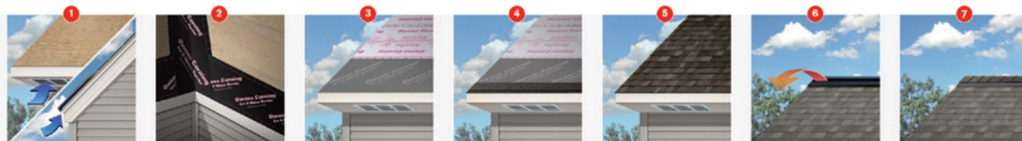
1 Help prevent heat and moisture buildup in the attic by allowing fresh air to enter the attic.
