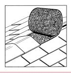
**STEP 4:** Install ridge cap shingles over top of vent using nails provided inside box. To ensure uniform look do not over drive nails. Ensure equal soffit ventilation.
